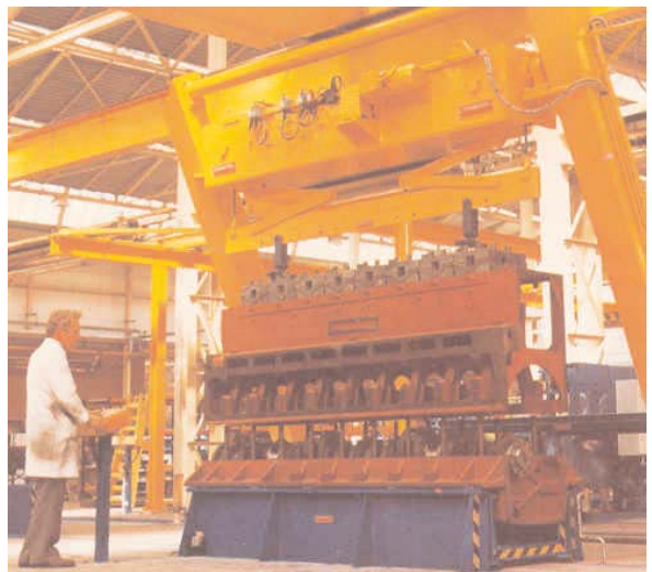
Figures 6, 7, and 8 Views of the 1979 track assembly of Blackstone E range Mark1 engines
