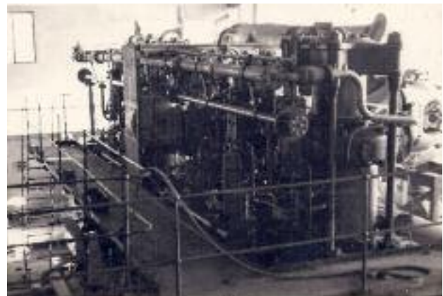
Figure 13 View of top of No 5 completed engine with covers omitted for better access
