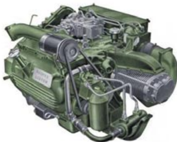
Figure 8: Illustration of the front end of a Rootes-Lister TS3 and the Roots blower
