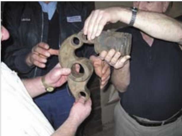
Figure 2: TS3 rocker arm and piston assembly
