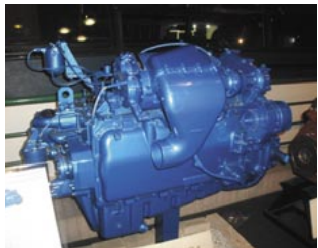
Figure 10: TS4 Stage II prototype engine with top mounted blower at the British Commercial Vehicle Museum in Leyland
