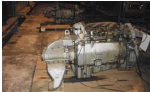
Figure 9: Two TS4 prototype Stage I engines at the Science Museum store (with end mounted blowers)
