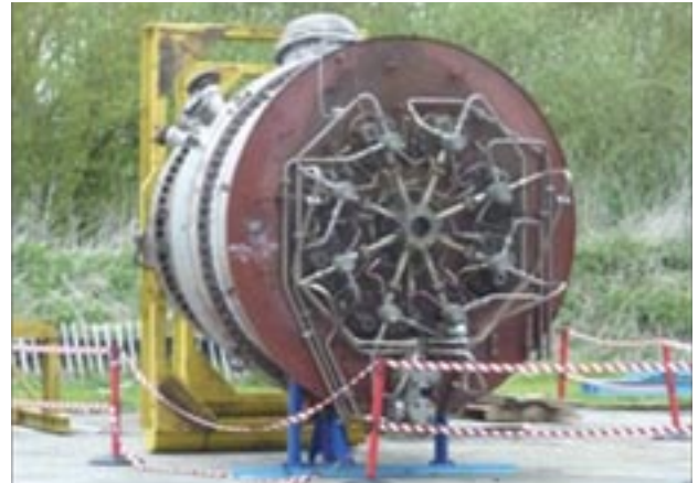
Figure 3: Gas turbine silo combustor ready for scrap or resale
