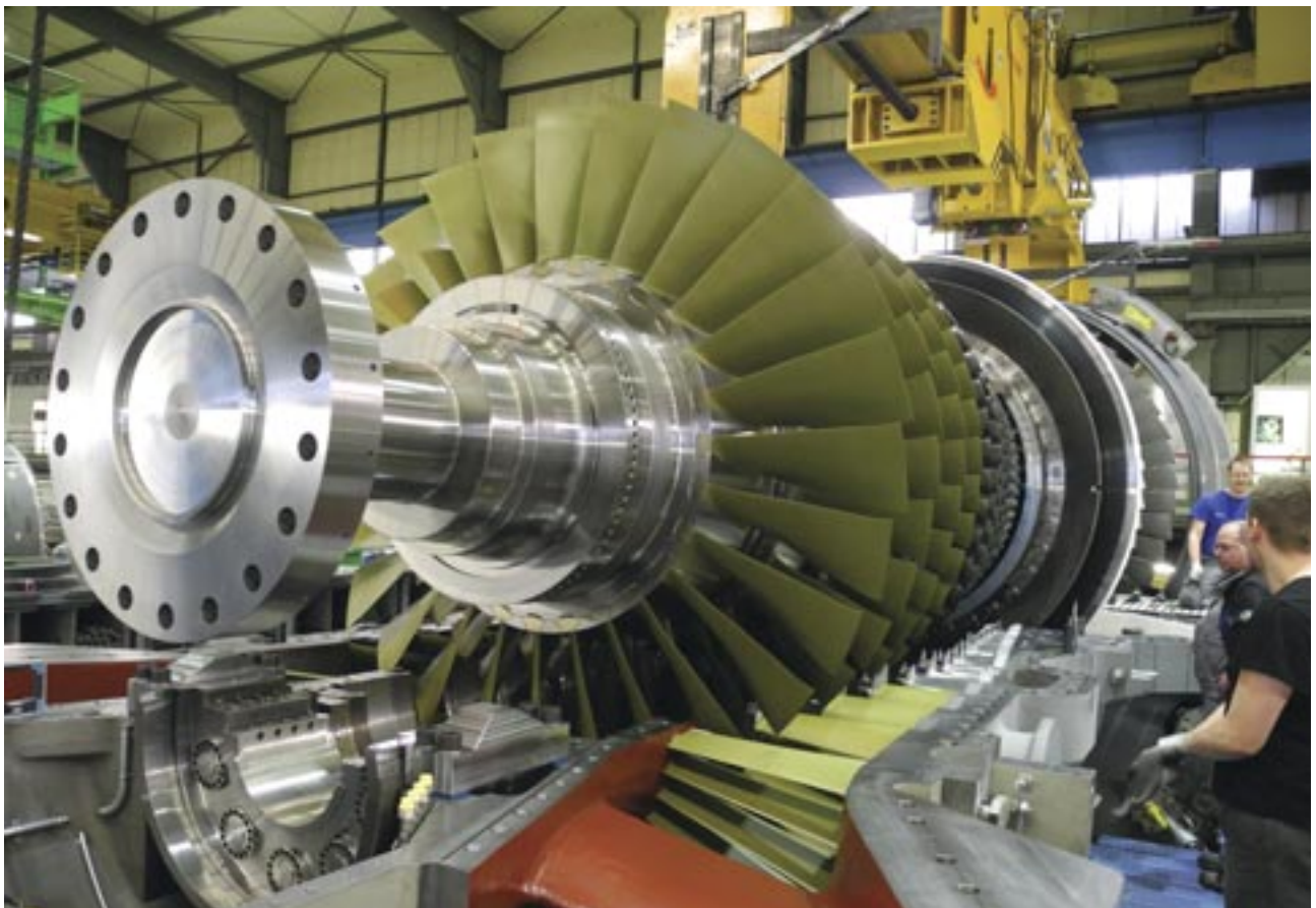
Figure 4: New SGT5-4000F in Siemens' Berlin assembly works
