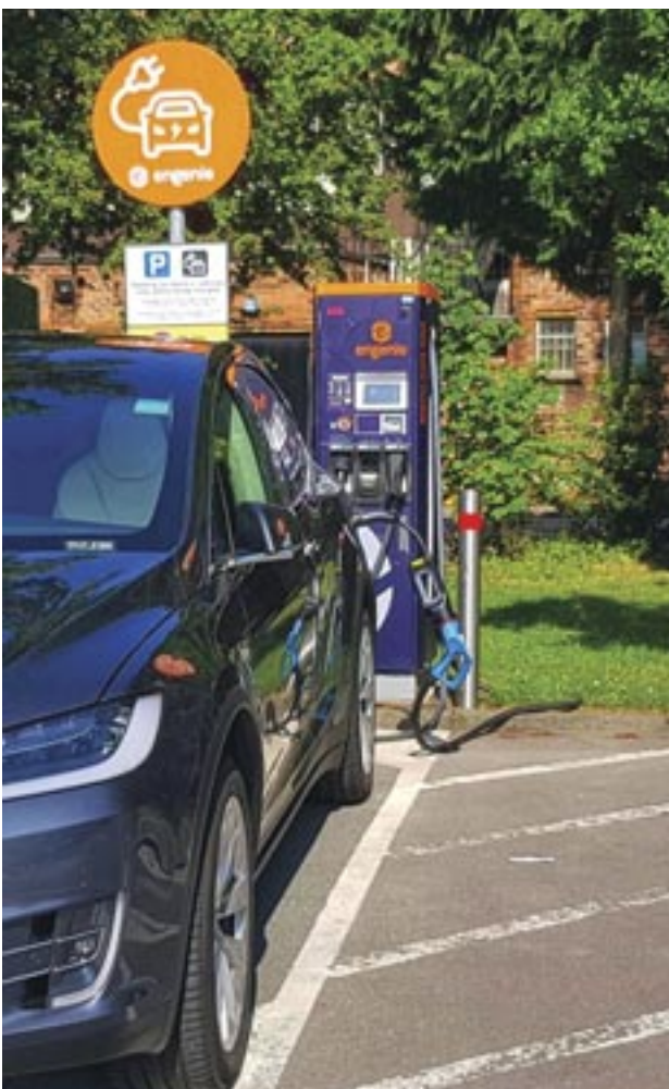
Figure 5: Our car charging at an Engenie 50 kW charger using a Type 2 socket converter attached to a blue CHAdeMO connector
