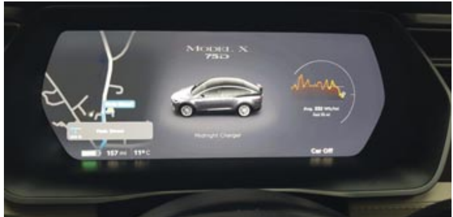
Figure 8: Steering wheel binnacle view showing immediate routing along with range and power usage
