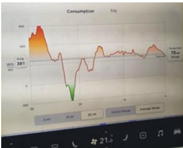
Figure 2: Car visual display showing power usage over the past 30 miles along with the projected range based on the average achieved
