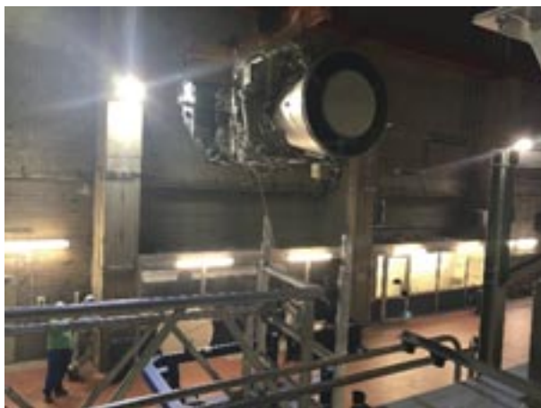
The core engine being hoisted to the platform
