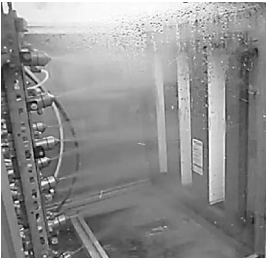
Figure 3: All the water droplets generated must impact the tested filter
