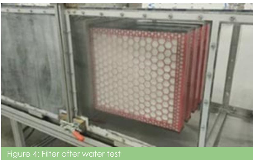
Figure 4: Filter after water test
