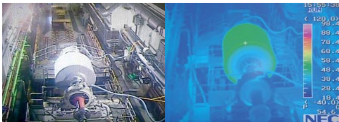
Figure 8 – Flywheel during factory balancing in the pit with experimental thermography on the right
